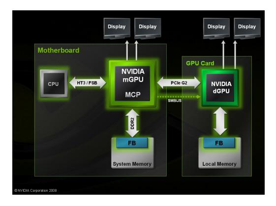
Figure 1. Hybrid SLI Block Diagram
